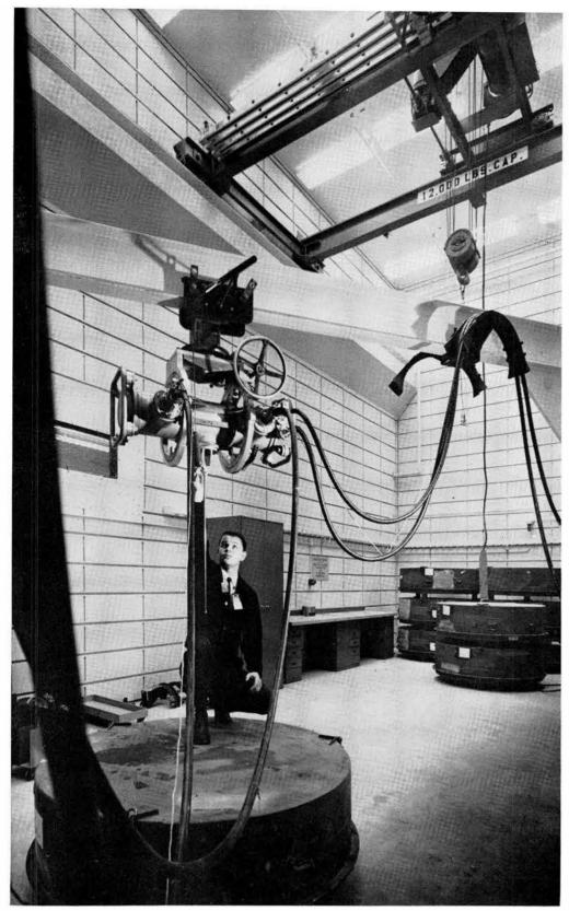
A 300-KV INDUSTRIAL X-RAY UNIT is being positioned by Dennis J. Adkins preparatory to examining a sealed parachute case. The high ceiling and overhead crane provide easy handling for large objects.
